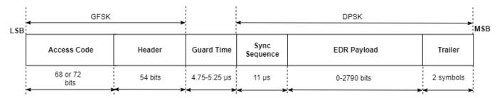
The format and modulation of the access code and the packet header fields are similar to that of BR packets. Following the header field, the EDR packets have a guard time in the range [4.75, 5.25]  $\mu$ s, a sync sequence (11  $\mu$ s), payload in the range [0, 2790] bits, and trailer (two symbols) fields.
