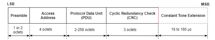
Each packet contains four mandatory fields (preamble, access-address, protocol data unit (PDU), and cyclic redundancy check (CRC)) and one optional field (constant tone extension (CTE)). The preamble is transmitted first, followed by the access address, PDU, CRC, and CTE (if present) in that order. The entire packet is transmitted at the same symbol rate of 1 Msym/s or 2 Msym/s.
