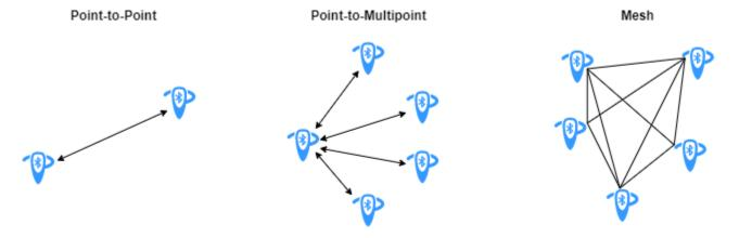
Devices using one-to-one communication operate in a Bluetooth *piconet*. As shown in this figure, each piconet consists of a device in the role of *Central*, with other devices in the *Peripheral* or *Advertiser* roles. Before joining the piconet, each *Peripheral* node is in an advertiser role. Multiple piconets connect to each other, forming a Bluetooth *scatternet*.
